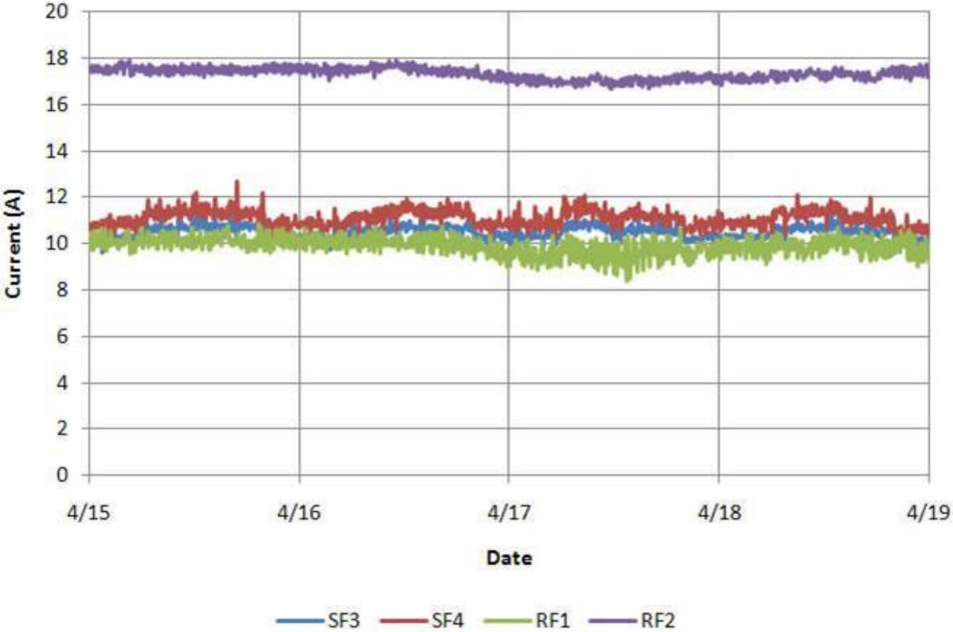
Figure 4.7 Supply and Return Fan Amperages for AHU-2
